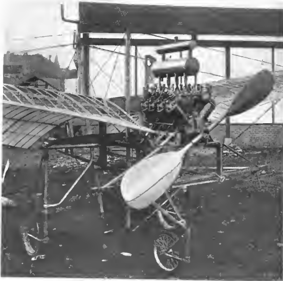
Fig. 3—Fifty-Horsepower Eight-Cylinder Antoinette Engine Mounted on Aeroplane to Drive Two-Bladed Propeller as Shown.
